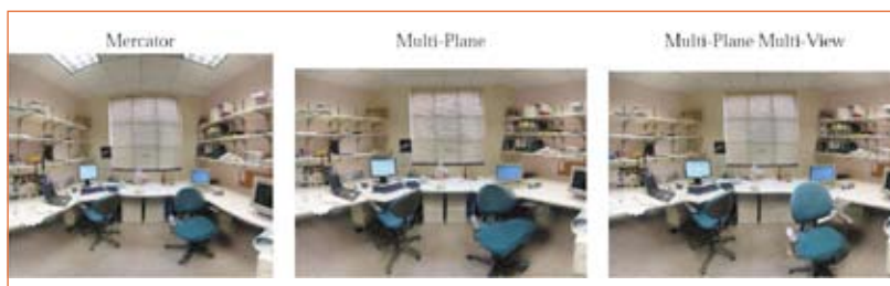
Figure 4. Multi-Plane Multi-View. The multi-plane projection rectified the background but the chair on the right got distorted. Using the Multi-View approach the chair is undistorted.
