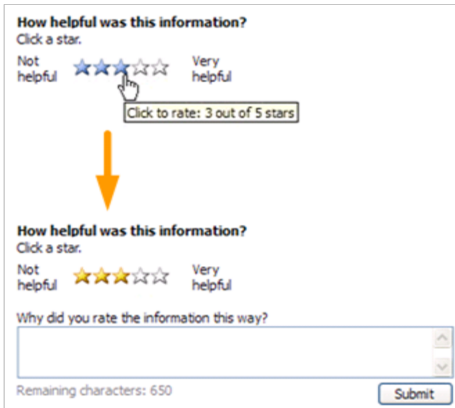
Redesign, Variant B (showing the two stages of the rating area, before and after the user has assigned the star rating)
